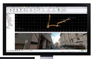
Work with trajectory, registered point cloud, and imagery
